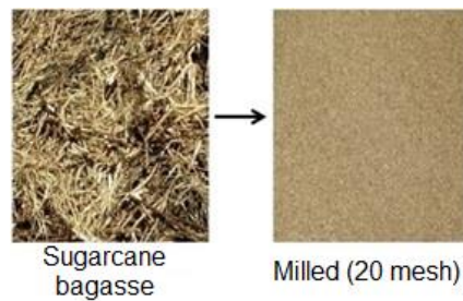
Figure 1. Sugar cane bagasse before and after milling (20 mesh).
