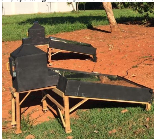
Figure 2. Dryer 1 (top) and dryer 2 (bottom) operating in an experimental field at the Federal University of Mato Grosso.
