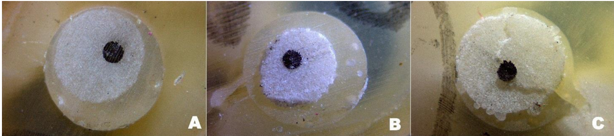
Figure 2: Representative stereomicroscopic images of fracture types (magnification: 10 X) (images from 100G). A) Adhesive fracture, B) Cohesive fracture and C) Mixed fracture.
