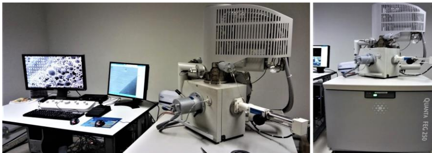
Figure 7: Scanning Electron Microscopy (SEM) – QUANTA FEG-250 With EDS microanalysis.
