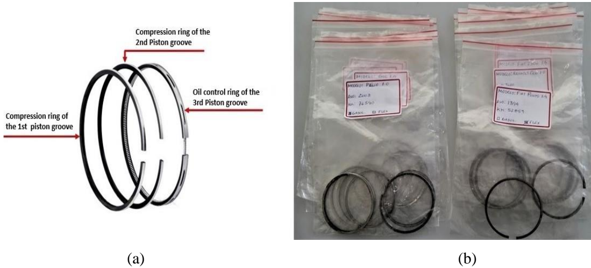
Figure 4: (a) - 1st Compression ring, 2nd compression ring and 3rd ring oil scraper. (b) - Samples acquired in an engine reconditioner.
