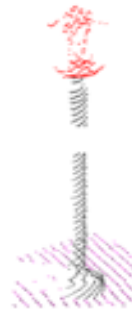
Figure 7: Example of a scanned object. Black = pole; red = top (glass ball lamp)
