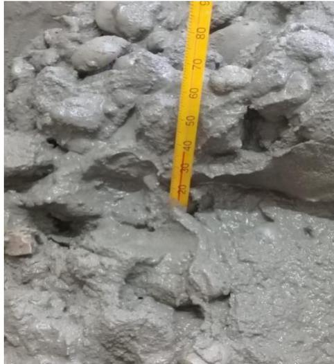
Figura 09 - Temperatura do concreto (Autor, 2020)
