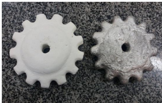
Figure 1: (a) polystyrene model and (b) aluminium part AA5052
