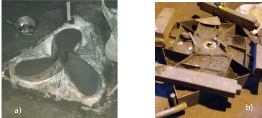
Figure 3: (a) Cast of a propeller. (b) Propeller Model (courtesy Fundição Barbosa Ltd.)
