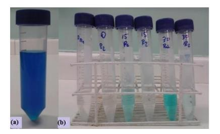
Figure 6. Methylene blue solution (20 mg/L): (a) original sample before enzymatic treatment;(b)Samples after 0, 15 and 30 minutes of continuous process from the effluents of each microreactors(R1and R2) operating in series.(R1
