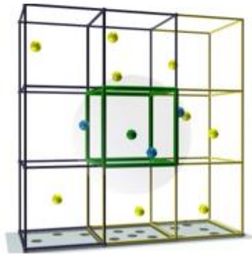
Figure 5. Example of a cell-list in a 3D grid, where N_x \times N_y \times N_z = 1 \times 3 \times 3 .
