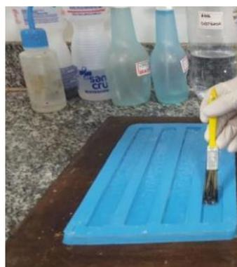
Figura 5. Molde de silicone conforme a norma ASTM D3039 (Autor, 2019).
