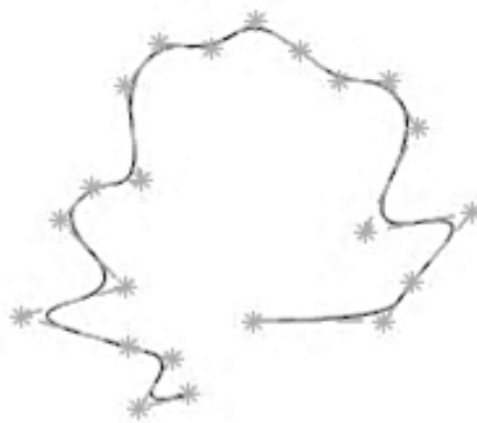
Figure 56: B-spline curve with 22 control points created by design model generation function with \pi = 1.25
