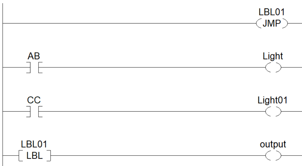
Fig. 5.5. Bypassing all the rungs between JMP and LBL instructions.
