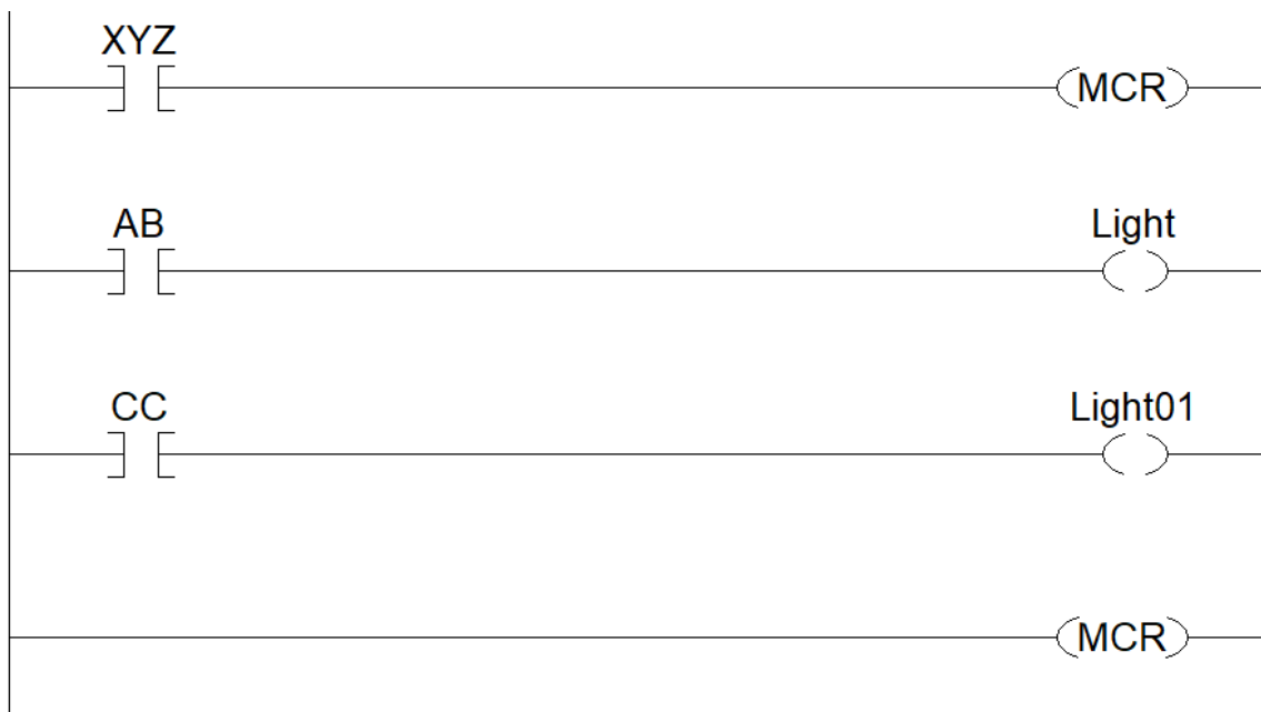
Fig. 5.2. Disabling outputs when MCR goes OFF.
