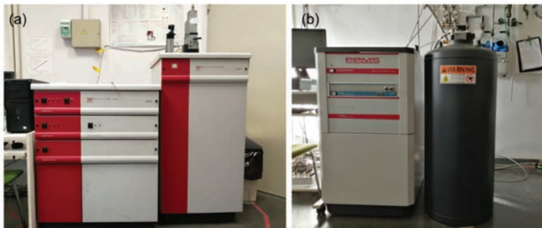
FIGURE 3.13: Views of the two different magnetometers used: (a) the Magnetic Property Measurement System (MPMS-XL) and (b) the Physical Properties Measurement System (PPMS), both located at the Low Temperature and Magnetometry Lab at ICMAB.
