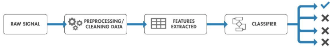
Figure 28: Feature Extraction process in raw signals and time series data for a ML classifier (taken from [87])
