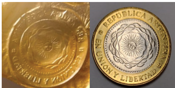
Figure 7. Hot-compression molding of the xylan/PEI of 50/50 mass ratio. The coin used to mark that the film is also shown. Image of coin: Copyright 2016, Banco Central de la República Argentina.
