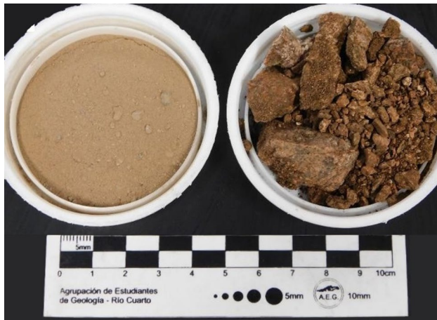
Fig. 5 Sediments used in batch tests to evaluate the release of As and F (Michelli 2020)
