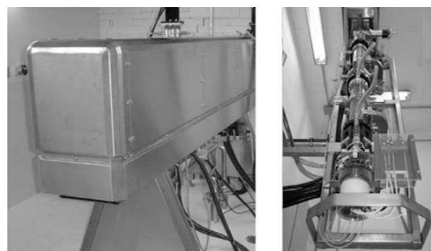
Fig. 6. MEVEX accelerator: left – general view; right – view with cover removed
