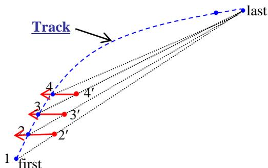
Fig. 5. Scheme of the algorithm for determining points along the track
