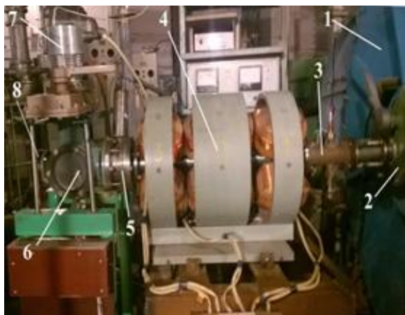
Fig. 2. Accelerator output: 1 – linear accelerator outlet; 2 – valve; 3 – Faraday cup; 4 – focusing triplet; 5 – induction transient sensor; 6 – chamber for irradiation of samples; 7 – turbomolecular pump; 8 – chamber with phosphor
