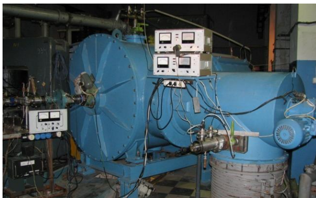
Fig. 1. Helium ions linear accelerator with output energy 4 MeV
