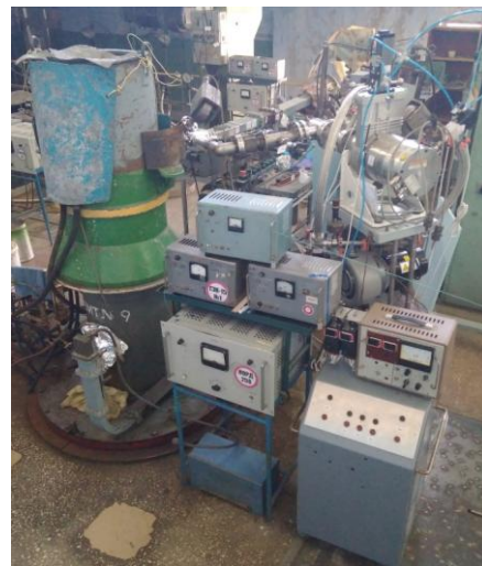
Fig. 6. Configuration of vacuum system during HV and RF training of klystron
