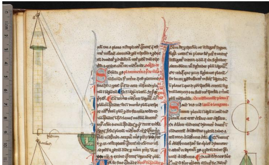
Figure 3. Quadrans vetus, Londres, Harley 3647, f. 59v. The use of instruments to grasp mathematical characteristics of objects, such as quantitative measures, is seen in this diagram displaying the measuring method of an object's height.
