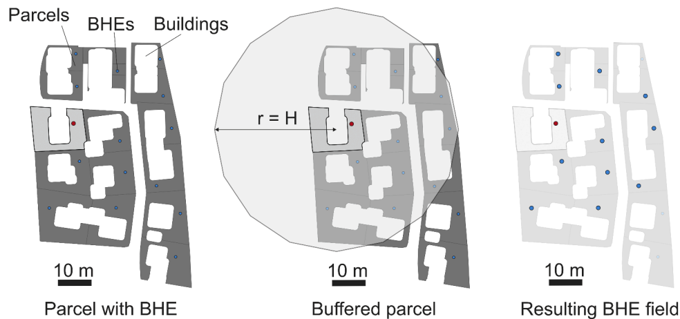
Fig. 1. Definition of borehole fields based on parcel buffering. The radius ( r ) of the buffer around a parcel equals the length ( H ) of the deepest borehole in the parcel considered. For the resulting borehole field, the steady-state g-function is calculated using the methodology described below. This is carried out for every parcel in the study area.
