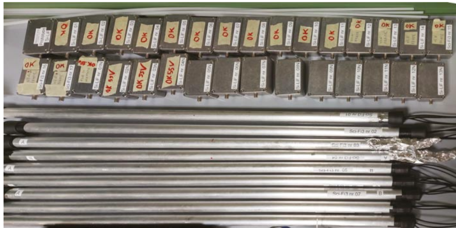
Fig. 1. – A set of SiLiF neutron (top) and SciFi gamma (bottom) counters developed in the MICADO project.
