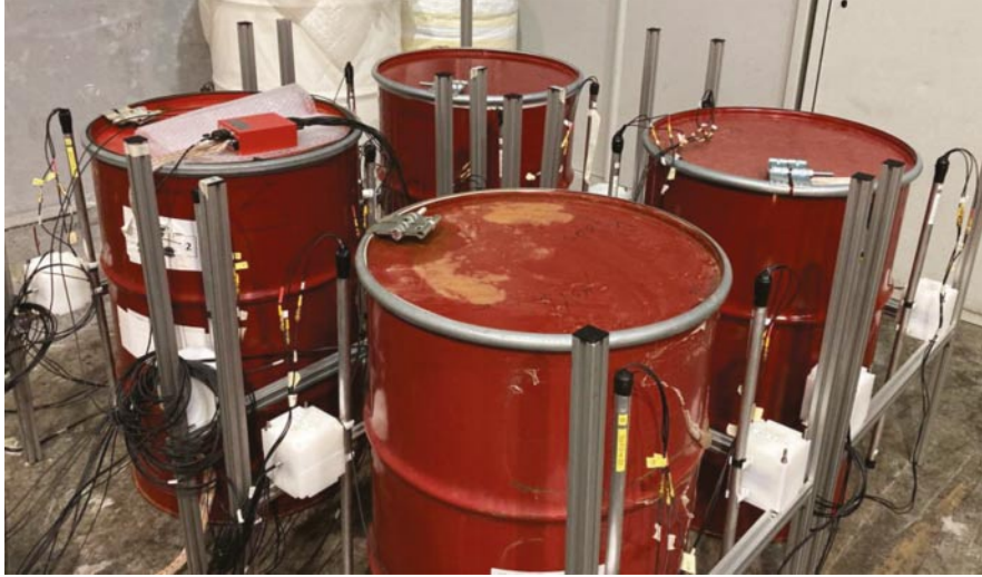
Fig. 2. – Four very low activity radwaste drums surrounded by 16 SciFi and 16 SiLiF radiation counters for gamma rays and neutrons respectively.
