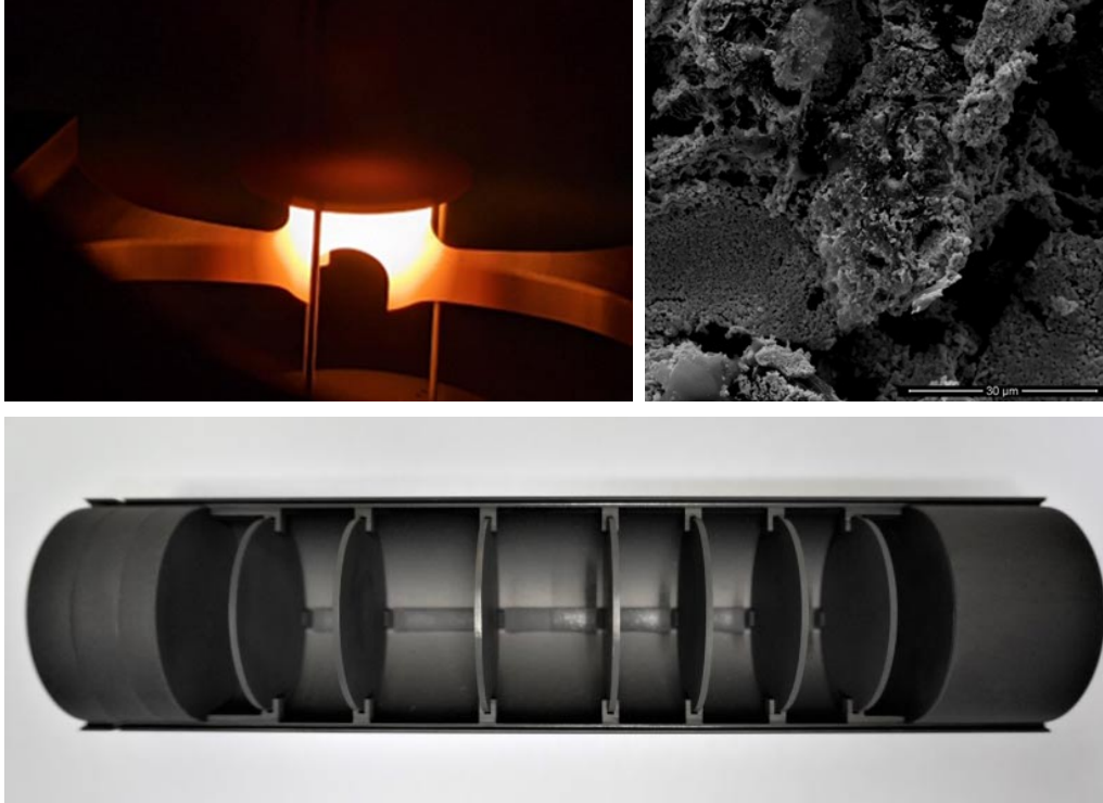
Fig. 5. – The target assembly including 7 UCx disks within a graphite container (on the bottom). A SiC target disk exposed to thermal gradients (top left), microstructure of uranium carbide containing carbon nanotubes (top right).
