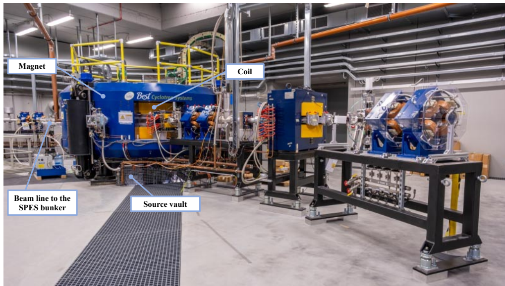
Fig. 2. – View of the Best ® 70p cyclotron: the SPES primary driver.
