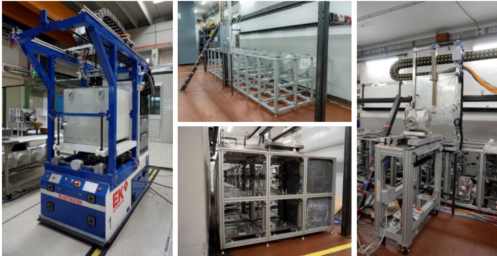
Fig. 7. – The Horizontal Handling Machine (HHM) during the tests in the SPES remote handling laboratory (left), the Temporary Storage System (TSS) during the construction phase prior to the installation (center, right).
