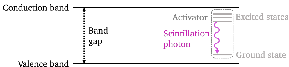
Figure 4.4.: An inorganic scintillator has a valence and a conduction band. Additional energy levels are made available in the band gap through doping the material with so called activators. These levels are usually passed when deexcitation of the atom from the conduction band occurs in the local impurity regions of the activators. The transitions between the added energy levels in the band gap are the scintillation transitions, that result in the emission of a scintillation photon, that is later detected by the CCD camera. Figure adapted from Reference 134.
