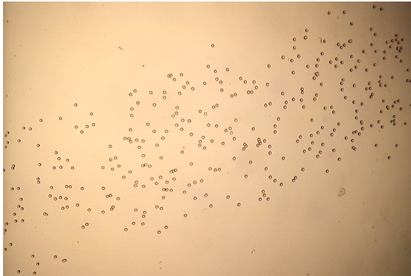
Figure 4.7.: Microscope image of one bar of the CR-39 after four hours of etching. Observed tracks are all the same size and can be attributed to deuterons ( \sim 0.49 MeV) with no presence of O^{8+} .
