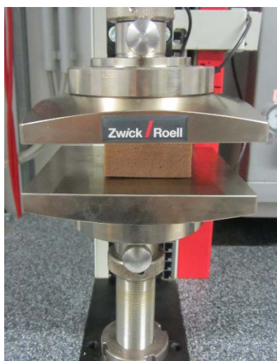
Figure S-7. Setup for deflection tests according to DIN EN ISO 3386-1.
