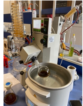
Figure 2- Rotavapor, the device used evaporation
