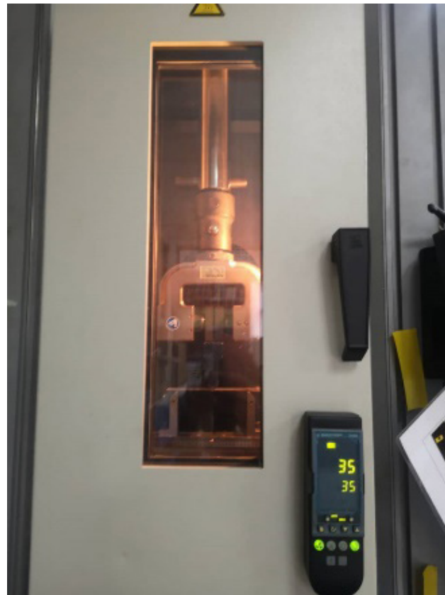
FIGURE 5. Flexural test at 35°C inside the heating chamber
