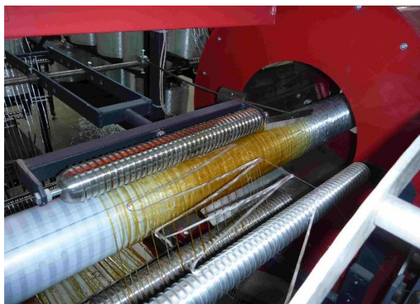
Figure 10: Pipe structure formation
