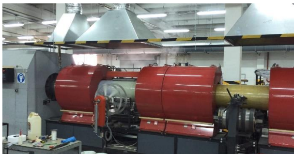
Figure 9. Equipment for continuous winding of pipes of standard size 300...800
