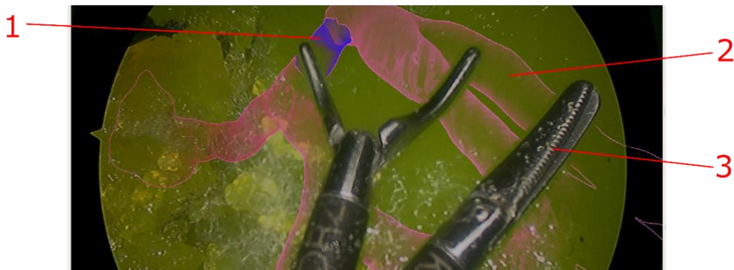
Figure 30: (1) Displayed target structure at vessel_01 for the user, (2) vessel_01 augmentation, (3) instrument – here the instrument segmentation is activated
