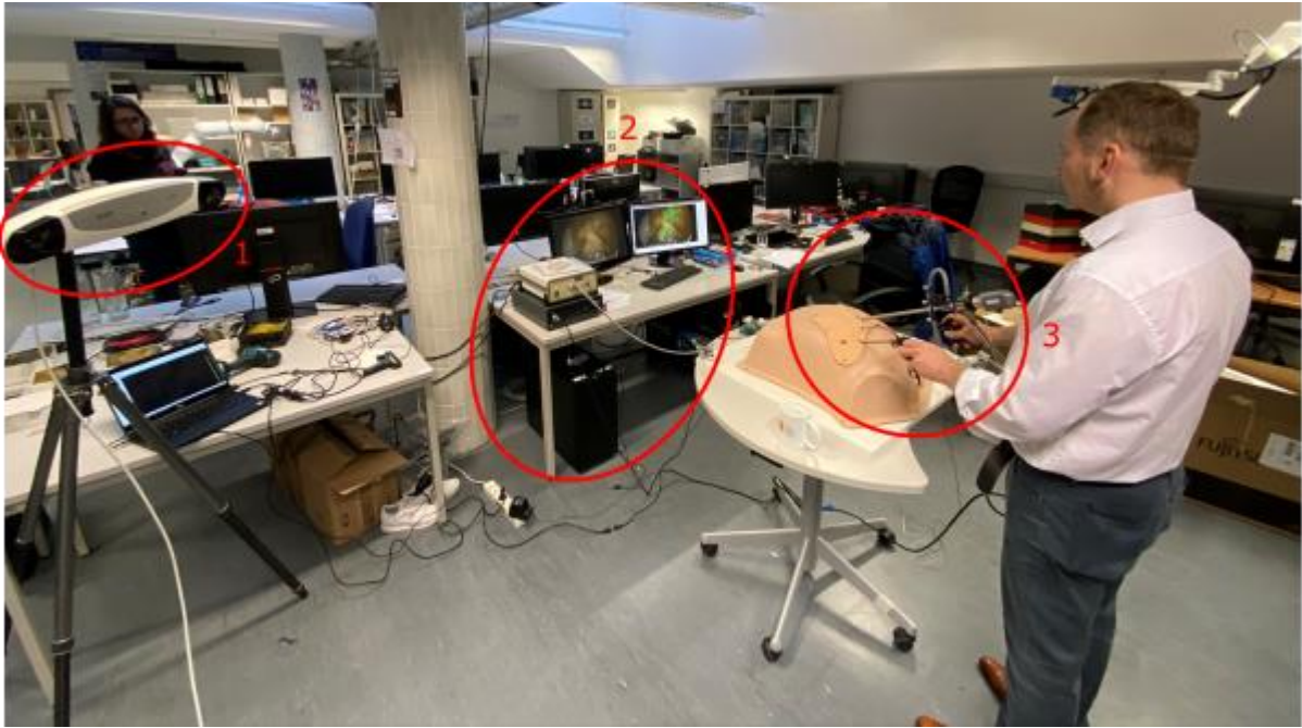
Figure 24: Setup of User Study II, (1) NDI infrared camera, (2) computer, endoscopy tower, two screens shown the endoscopic camera image with and without augmentation and (3) the endoscope and laparoscopic trainer
