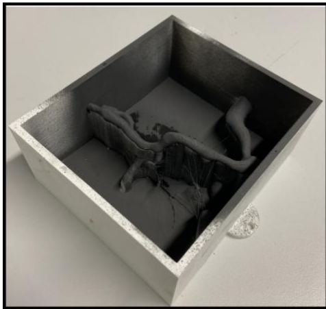
Figure 29: (Left) The graphite coated vessel box and (right) circuit diagram of the instruments, vessel box and USB-Oscilloscope
