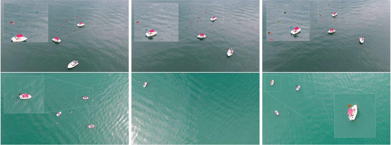
Figure 2: Common fragmentation and reidentification errors (here ReIDTracker-Sea ). Top: The detected swimmer in the first frame is lost in one of the next frames due to a heading angle change and is assigned a new ID when it is re-detected in a later frame. Bottom: A boat is not re-detected re-entering the scene after having left it. This may be caused by the great similarity between the different boats.
