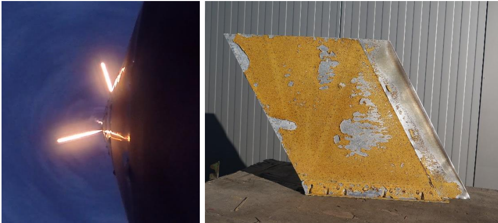
Figure 2: Thermal load on fin leading edges after 2 nd stage burn of DLR MORABA sounding rocket vehicle (left) and 2 nd stage fin with steel sheet metal leading edge and ablative TPS recovered after VSB-30 flight operation
