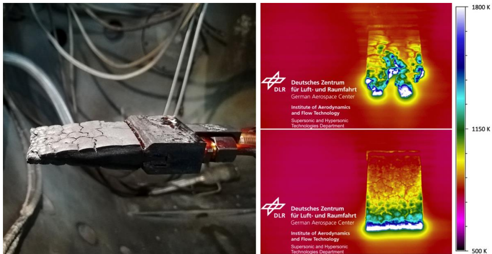
Figure 9: Test specimen after testing (left), thermographic images of oak (top right) and TUD-WBM-2 (bottom right) at 60 s
