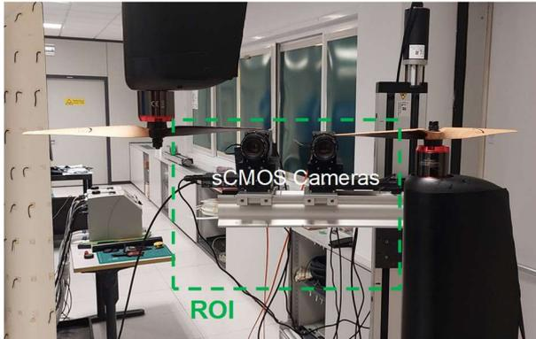
Figure 3 PIV set-up for tandem case in CIRA
