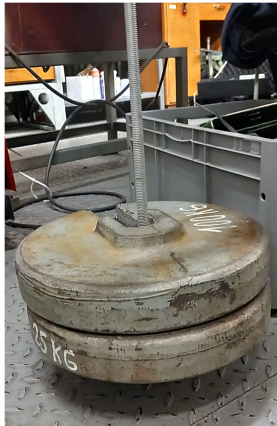
Figure 17. The force of 522.5 N applied to the clutch lever.
