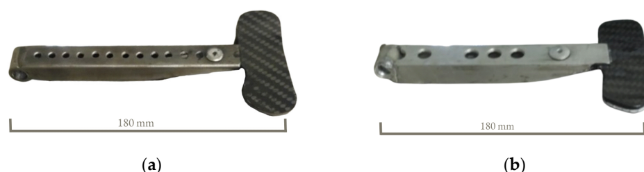
Figure 6. Already existing clutch levers: (a) the clutch lever made from steel and carbon fiber plate; (b) the clutch lever made from aluminum alloy and carbon fiber plate.
