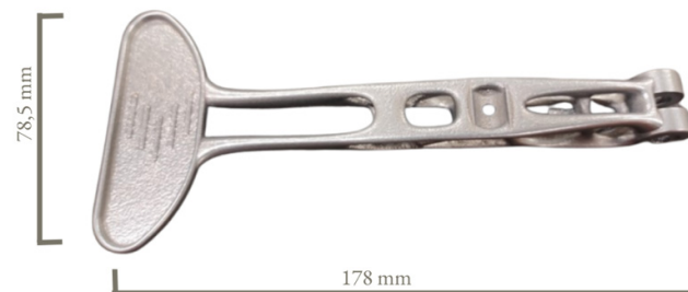
Figure 21. SLM-printed clutch lever, AlSi10Mg.
