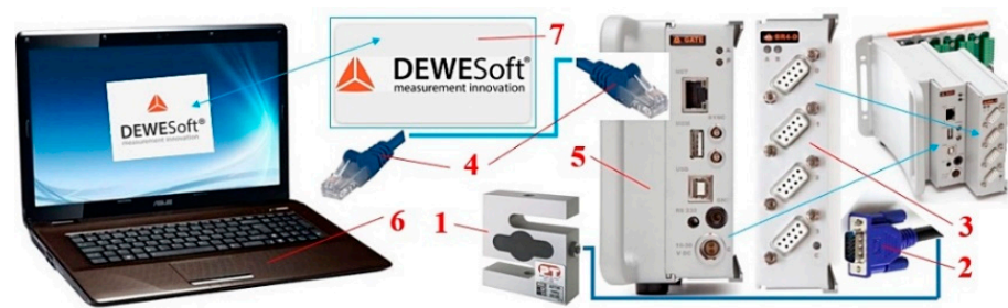
Figure 4. Measuring chain for the experimental measurement of conveyor belt tensile force: 1—load sensor; 2—D-sub plug; 3—measuring module BR4D of the strain gauge apparatus DS NET; 4—network cable; 5—gateway module DS GATE; 6—laptop; 7—software DEWESoft X2 SP5.
