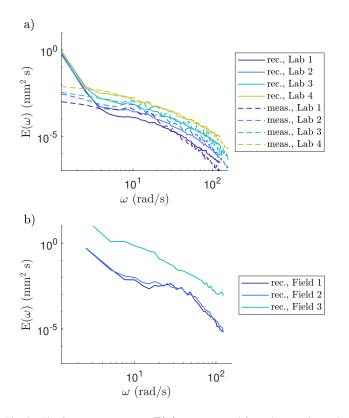
Fig. 9. The frequency spectrum,  $E(\omega)$ , reconstructed from the experimental data. (a): from laboratory data; (b): from field data. (dashed lines): frequency spectrum of the surface fluctuations measured with wave gauges.
