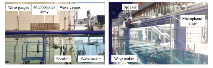
Fig. 4. Photographs of the experimental setup with the wave tank in the LVV facility at the University of Sheffield.
