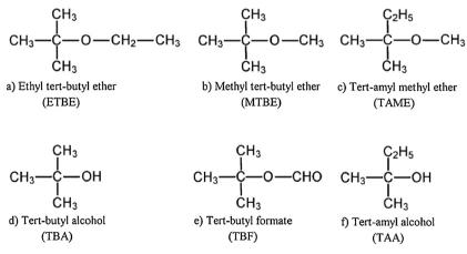
Fig. 1. Molecular structure of ETBE, MTBE and TAME (a-c) and their major metabolic intermediates (d-f), reproduced from Kharoune et al (2001b).
