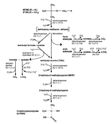
Fig. 2. Proposed aerobic pathway for biodegradation of MTBE and ETBE to 2-HIBA, reproduced from Müller et al (2007).
