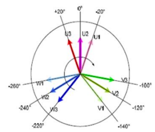
Figure 7: Triple three-phase machine windings from [45]
