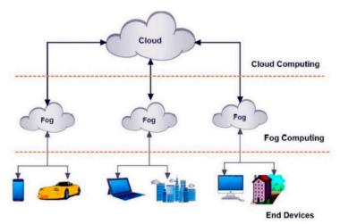
Figure 3. Fog computing is an expansion of the cloud but closer to end devices [25].
