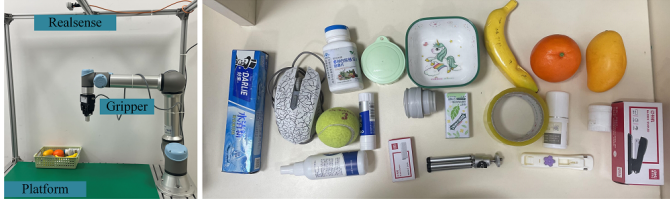
Fig. 12. The built low-light robotic grasping system and objects to be grasped.
