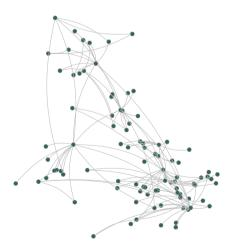
Fig. 3. Nationwide backbone network. Nodes are network elements distributed geographically across the country. Exact geographic location of the nodes has been randomised.
