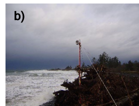
Figure 1: Photo of the mounted Lidar monitoring a single cross-shore line of the revetment at low tide, a) and high tide b). c) Photo of particle tracking survey using RFID detection and GPS.
