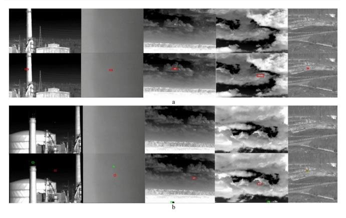
**FIGURE 6** Poor results of IC-SDDNet. (a) The first line shows missed detection results, and the second line shows the actual target positions with red bounding boxes. (b) The first line shows the original images. In the second line, the red bounding boxes indicate correct detections, and the green boxes indicate falsely detected background clutter.
