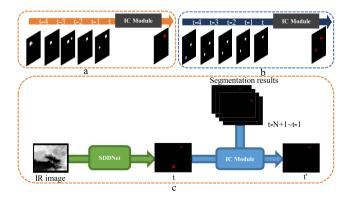
**FIGURE 2** (a) Eliminating false alarm (FA) areas. (b) Filling in missed targets. (c) The information processing of IC-SDDNet.
