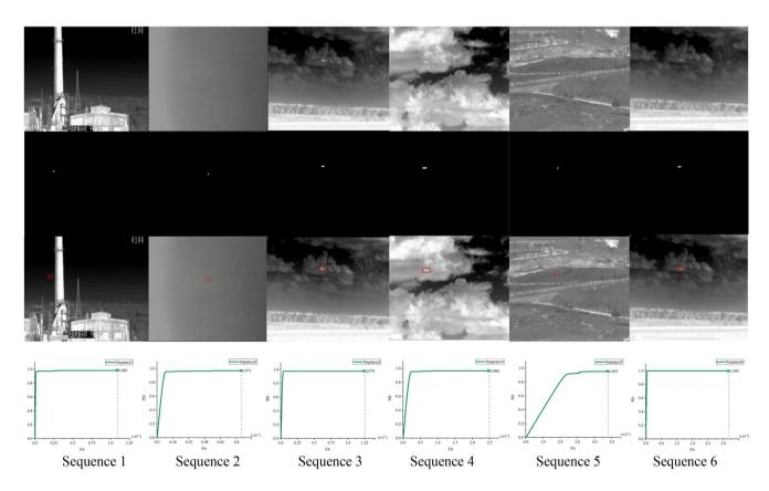
**FIGURE 4** Typical results of SDDNet. The first line is the original infrared image, the second line is the image segmentation result, the third line is the detection result where target is indicated with bounding boxes, and the fourth line shows the receiver operating characteristic (ROC) curves with respect to six sets of data.
