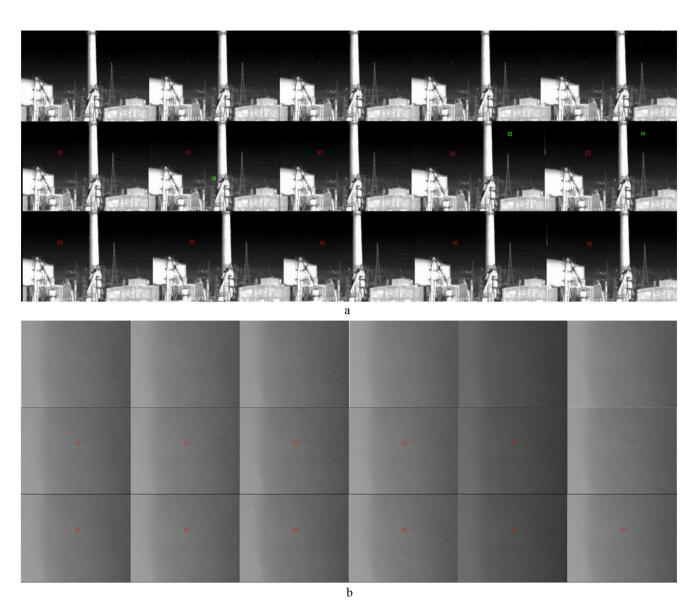
**FIGURE 5** Results of IC-SDDNet and SDDNet. (a) Reduction in false alarm (FA) rate. (b) Filled in missing detection. The first line is the original image, the second line is the results of SDDNet, and the third line is the results of IC-SDDNet.
