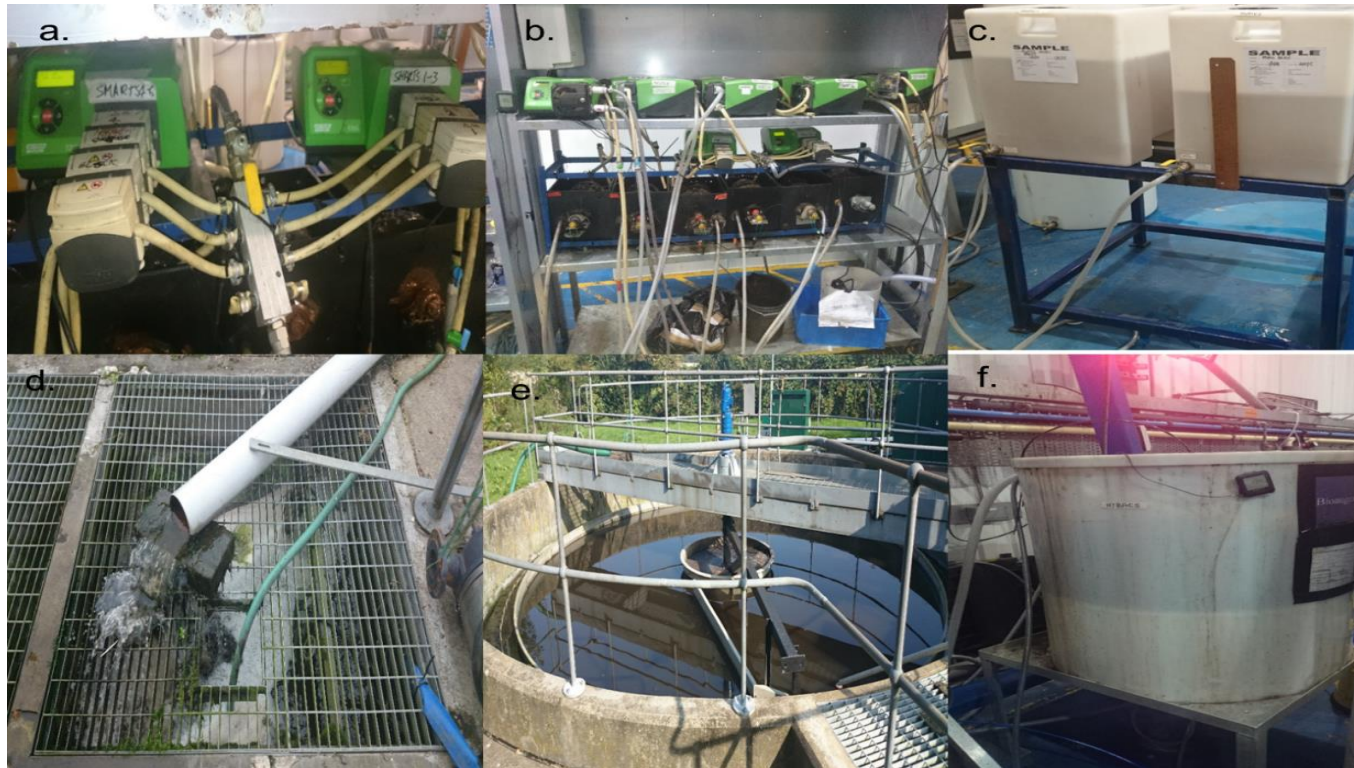
B.4.1 Experimental setup for Chapter 6 a. calibrated flow splitter for influent feed, b. Recycle pumps top of image and hybrid RBRs bottom, c. Feed tanks for HS and FE, d. FE sample point, e. HS sample point from bottom of clarifier, f. pilot scale ASP reactor.
