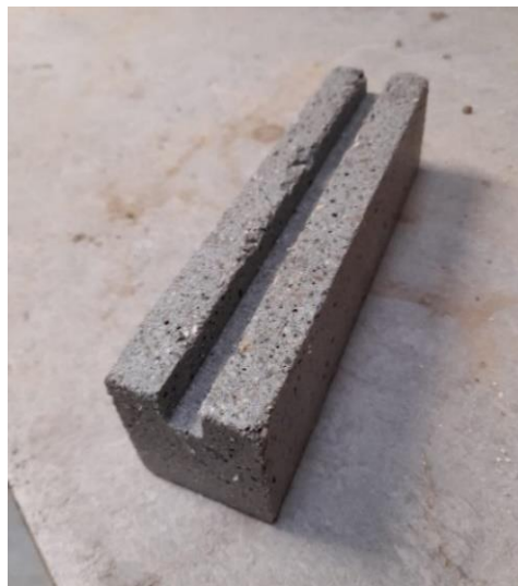
Fig. 3. Concrete prisms to be retrofitted.
