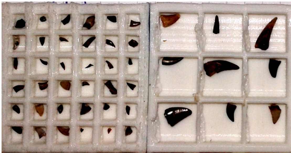
Fig. 2.7. 3D printed specimen holder trays for CT scanning of microvertebrate specimens. Specimen trays are 4 x 4 cm in size with locator boxes either 0.5 x 0.5 cm (left tray) or 1 x 1 cm (right tray) allowing either 36 or nine individual specimens to be located per tray. Trays are stacked six high for scanning.
