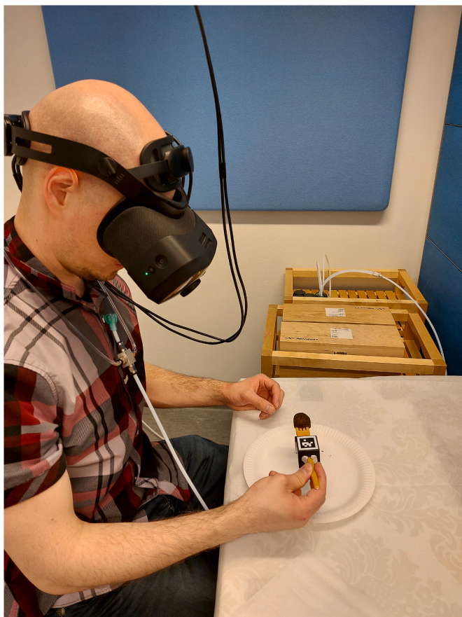
Fig. 2. Augmentation technologies in action at a study visit. Participants wore a head-mounted extended reality display for visual augmentation and an odor necklace with the green tube outlet positioned towards the nasal area for olfactory augmentation. The haptic augmentation was created by an electromagnetic field between actuators embedded in the table surface under the tablecloth and pellets inside the cube attached to the fork.
