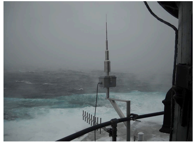
Fig. 9. Rotating multicylinder mounted on Mt. Desert Rock lighthouse (Jones and Andreas, 2014).
