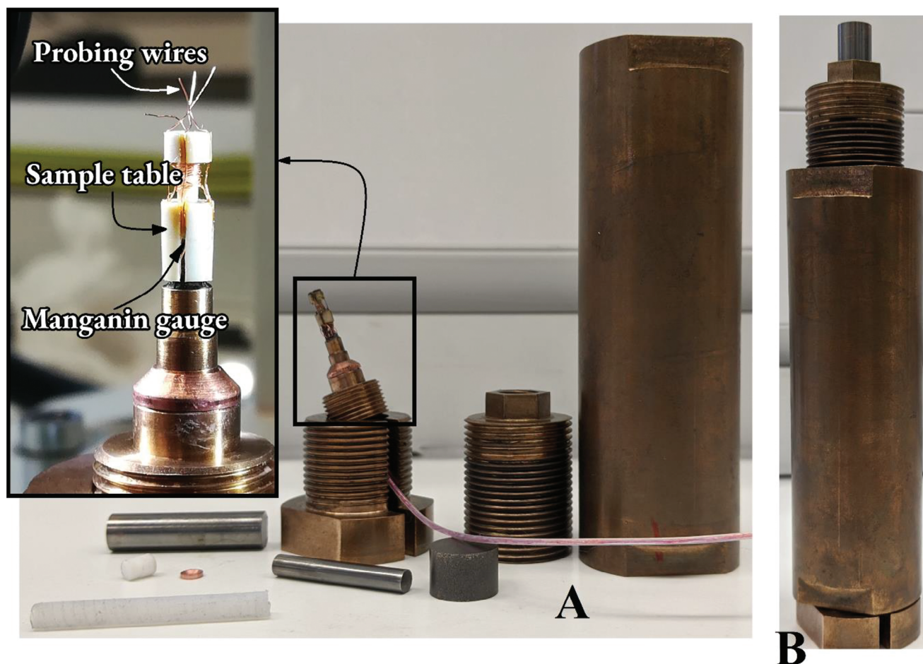
Figure 4. P-C cell with A – disassembled and B – assembled configuration. The zoomed-in insert (left) illustrates the feedthrough plug with a sample table.
